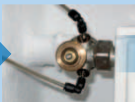
Insert the measuring probes
