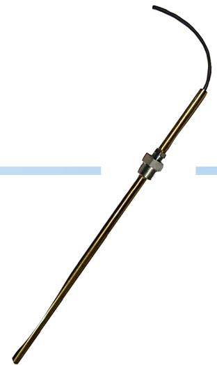
The sensing element of the probe consists of a stainless steel encapsulated thermistor of PTC-type. PTC = positive temperature coefficient, this means that when the thermistor is connected to intrinsically safe current and thereby is heated, it increases its resistance as the temperature in the thermistor gets warmer. Since the thermistor only can reach its warm temperature when it is in air the connected electronic unit can determine if the probe is in air, gas or liquid.
