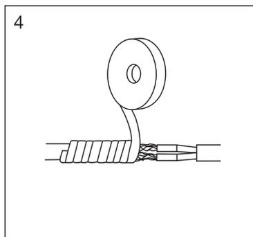
Fix the joint location with electrical tape, insulating tape or equivalent. Protect the power cord in the ground with conduit or the like.
