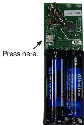
Hold down the button and insert the battery. When both LEDs are lit for about 1 second at the same time, release the button now. Both LEDs show flashing, 10 seconds in between. After about 10 minutes a return to normal operation.
