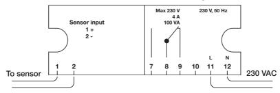
ES 21 with voltage free output for alarm panel etc.
