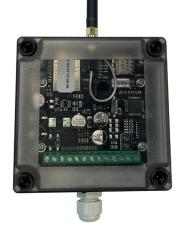
SMS-Alarm 4G is our new generation 2G/4G alarm transmitter that can be programmed entirely via the Internet. Via a web page, all settings are made such as managing receivers, configuring inputs, etc.
